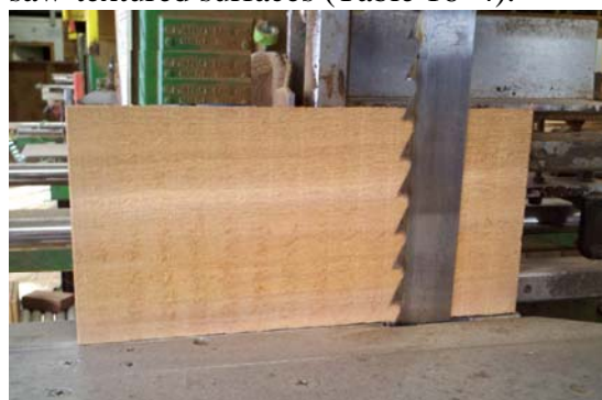
Picture of cross grain sawing of shingles
