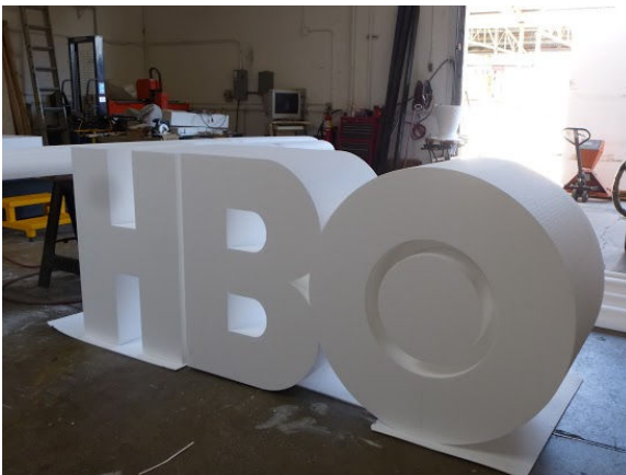
High-Density EPS foam Dimensional Letters before and after applying Polyurea coating
