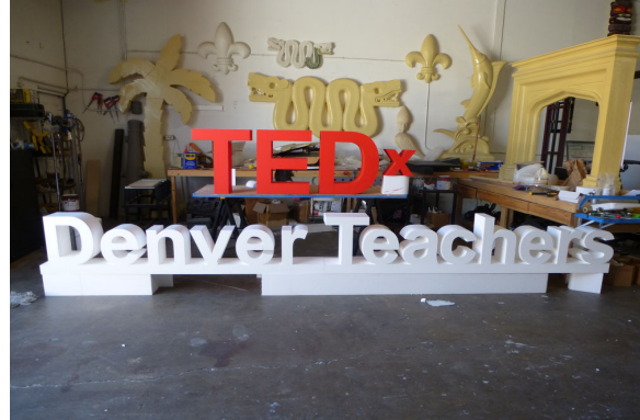
These TED Conference Dimensional Letters were cut with a CNC hot wire foam cutter, coated with polyurea and painted
