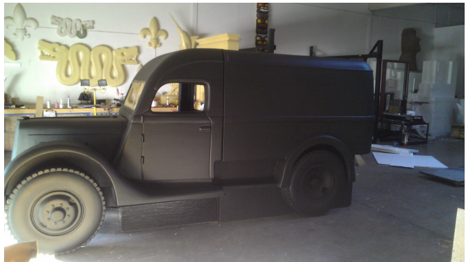
1937 Renault Truck Replica Machined from high-density EPS foam, coated and painted
