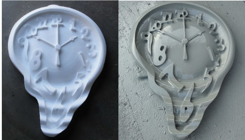
EPS foam prop before and after polyurea coating
