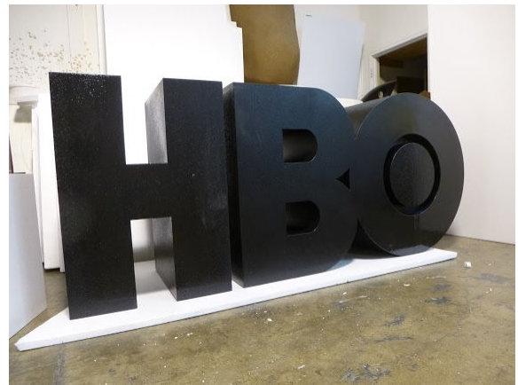
High-Density EPS foam Dimensional Letters before and after applying Polyurea coating
