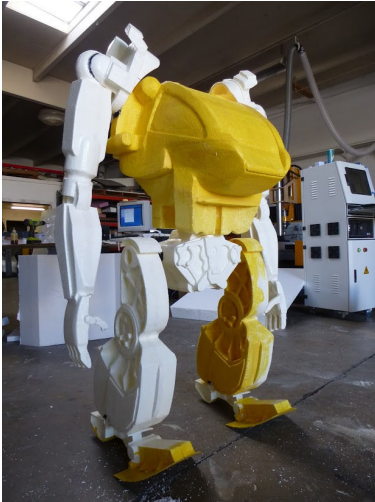
Avatar Robot 3D Prop created for a movie set. On the left – EPS machining and coating with prime, in the middle – coated with hard coat polyurea, to the right – spray painted
