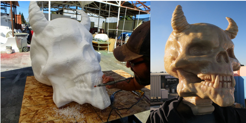
Skull Head – Machined from EPS, hand carved and coated in fiberglass
