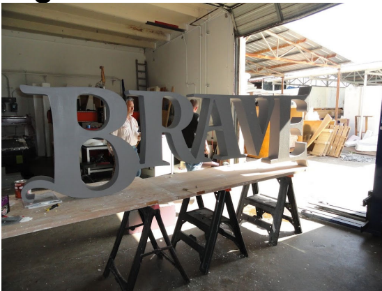
Disney Pixar Movie Sign created with our hot wire cutter, coated and painted
