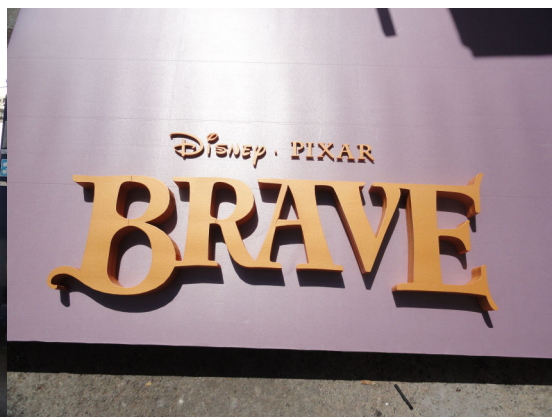
Disney Pixar Movie Sign created with our hot wire cutter, coated and painted
