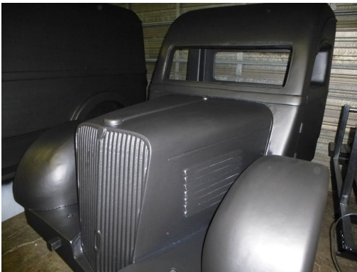
1937 Renault Truck Replica Machined from high-density EPS foam, coated and painted
