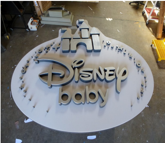
This logo sign was hot wire cut, then coated, painted and glued on Plexiglass
